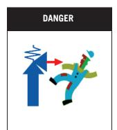
Never face the outlet of a valve when it is discharging as this may result in serious personal injury or death. There should be zero pressure at the valve inlet prior to commencement of any work which is to be performed.
